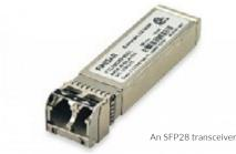
SFP28 stands for small form-factor pluggable 28. It is the third generation of the SFP interconnect systems designed for 25Gbit/ sperformance per the IEEE 802.3by specification. It has evolved from 100 Gigabit Ethernet, which is typically implemented with 4 × 25 Gbit/s data lanes. SFP28 is backwards compatible with SFP+ ports. The corresponding fiber optical plug is the LC-duplex connector.
