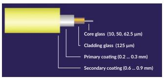
The modes in multimode glass fibers with a gradient index profile run in a wave shape around the fiber axis, which provides for an extensive compensation of signal delay differences. This glass fiber type has an attractive costbenefit ratio, and has established itself as the standard fiber for high-speed connections over short to medium distances.
