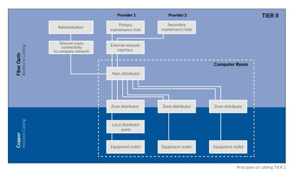
Backbone cabling and horizontal cabling at the Tier II level are also in a star topology and not redundant. Redundancy must be planned for active network components and their connections. Network operation may only be interrupted at specified times or only minimally during peak hours of operation.
