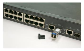
030.6125 SFP transceiver plugged into an switch port
