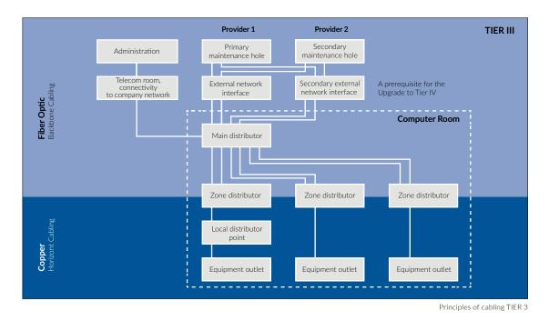
Backbone cabling and active network components are configured redundantly in a star topology at the Tier III level. Network operation must be maintained without interruption within specified times and during peak hours of operation.
