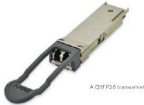
QSFP28 is the next generation of the QSFP form factor, delivering 100GbE. QSFP28 may also be used to break out a single 100GbE switch port into four individual 25GbE server connections with SFP28 transceivers. The corresponding fiber optical plug for singlemode devices is the LC-duplex connector, and for multimode the MPO8 or MPO12.
