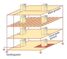
Earthing system as a mesh structure
