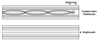
Only one light path exists in single-mode glass fibers. The reason for this is their extremely thin core diameter of 9  $\mu$ m. As a result, no multi- path propagation with signal delay differences between modes exists in these fibers. The advantage of this is that single-mode glass fibers can maintain extremely high transfer rates over long distances.
