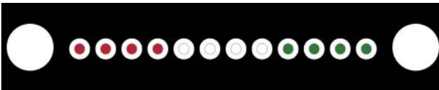
12-fiber MPO connector. Color highlighting shows fibers for sending (red) and receiving (green).
