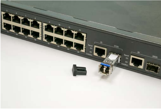
030.6125 SFP transceiver plugged into a switch port
