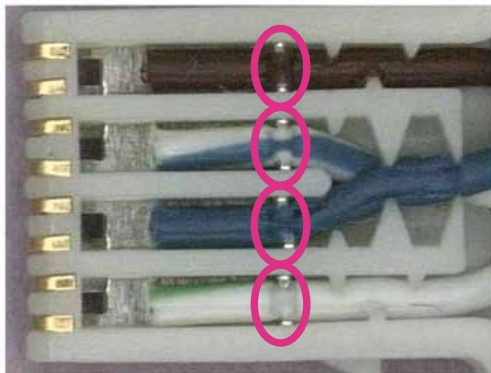
Figure 4: Use of RJ45 plug insert from R&M with IDC technology
